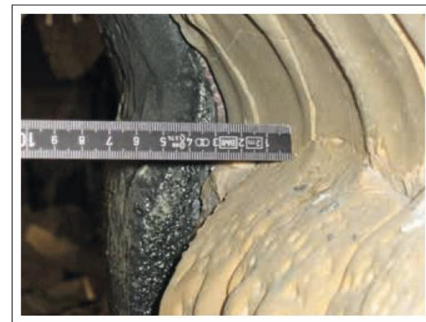
Figure 7. Wear of AZS overcoating tiles (white) in the foreground and chrome corundum overcoating tiles (black) in the background, both after 2 years application.
